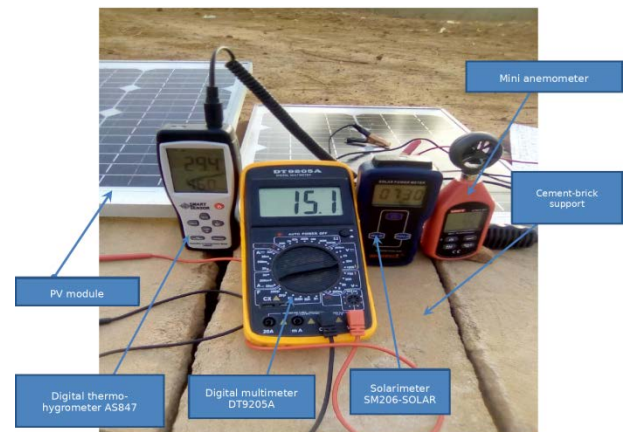
Figure 2. Experimental measurement setup used at the Dosso site. The instruments shown include the AS847 thermo-hygrometer, DT9205A digital multimeter, SM206-SOLAR solarimeter, and UT363 BT mini-anemometer. Photograph from the authors' 2021 field campaign, previously published in Baare Ali et al. [10] and reproduced under the Creative Commons Attribution (CC BY) License
