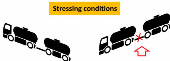
Figure 1. Point of failure: the locking mechanism of a tractor trailer
