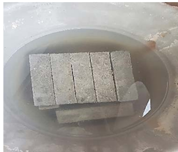
Figure 10. Curing of Specimens at 7 and 28 Days
