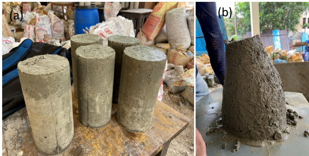
Figure 5. Constructed Sludge-concrete Cylinders (a) Final cylinders (b) Slump test
