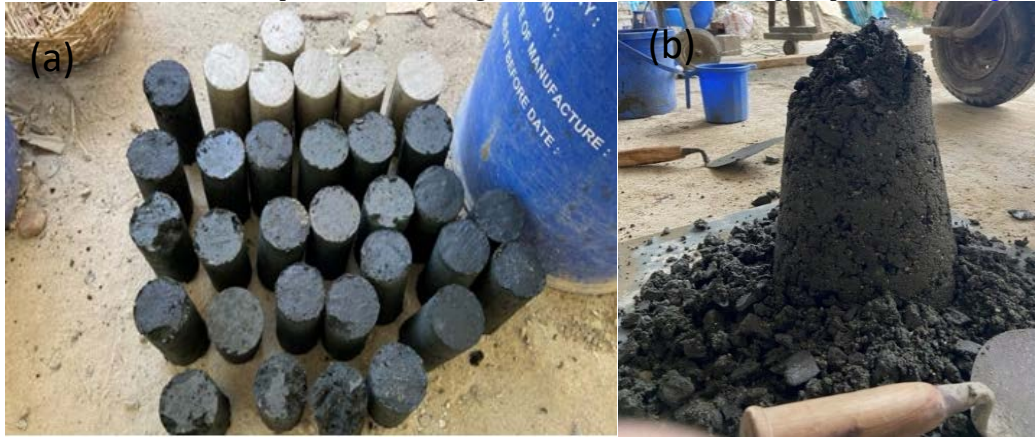
Figure 4. Trial Phases (a) Weak Concrete Cylinders (b) Slump Test
