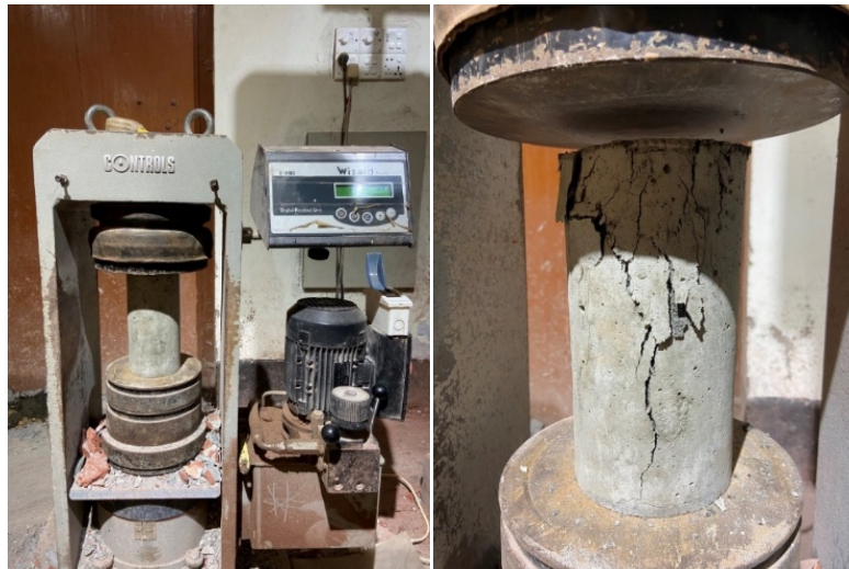
Figure 7. Compressive Strength Test of Concrete Cylinder
