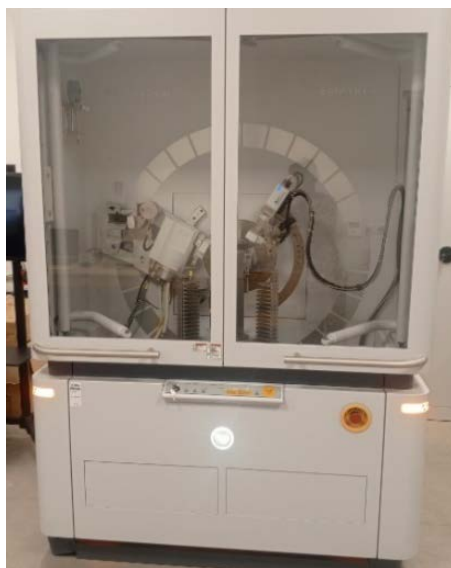
Photo 5: Powder diffractometer (PANalytical Empyrean from X-TechLab)
